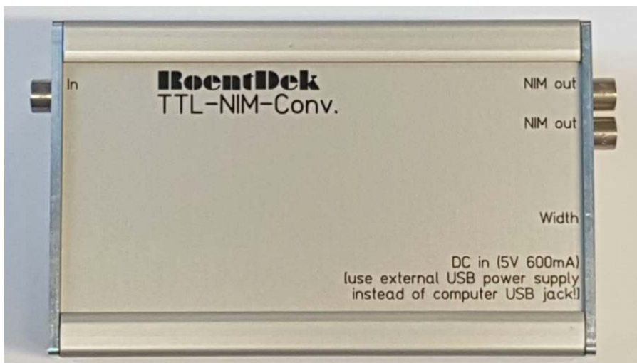
Figure: RoentDek LA1 configured as TTL-NIM converter.
